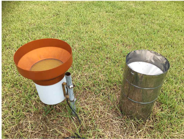
Fig. 3. The automatic measurement of precipitation (0.1 mm tipping Bucket Rain gauge, left) and manual precipitation gauge(right).
