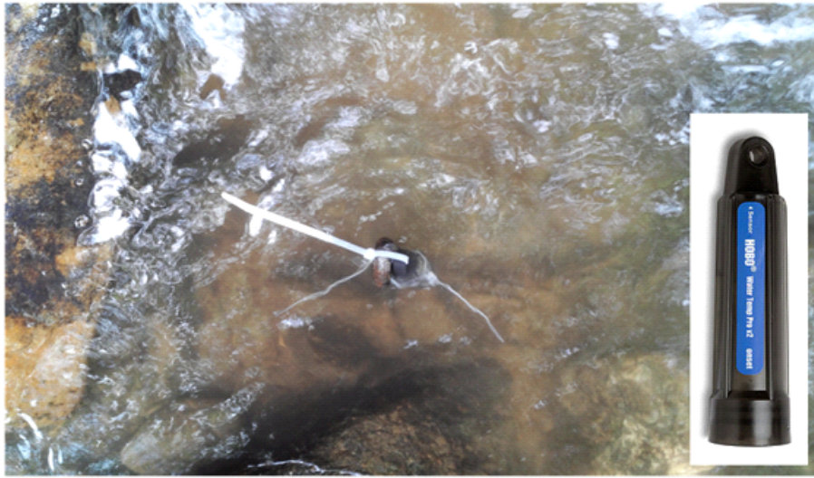
Fig. 2. Photos of the water temperature sensor installation at point 1.
